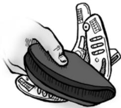
Attach the replacement pads. Fold the pads in half with the dull side out next to the velcro (the shiny side goes against the skin); then center the pad in the white shell.
