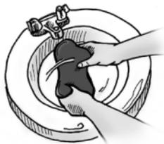
Wash the pads with mild facial soap and water. **DO NOT** use bleach or harsh detergents. Thoroughly rinse the pads with clean water. Wring out the excess water and squeeze in a towel. Lay the pads out flat to air dry. It should take less than 60 minutes for them to dry.
