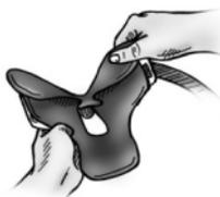
Peel the soiled, blue pads off. Look carefully at the shape as you remove them so that you can reposition the clean pads properly. The pads attach with velcro.
